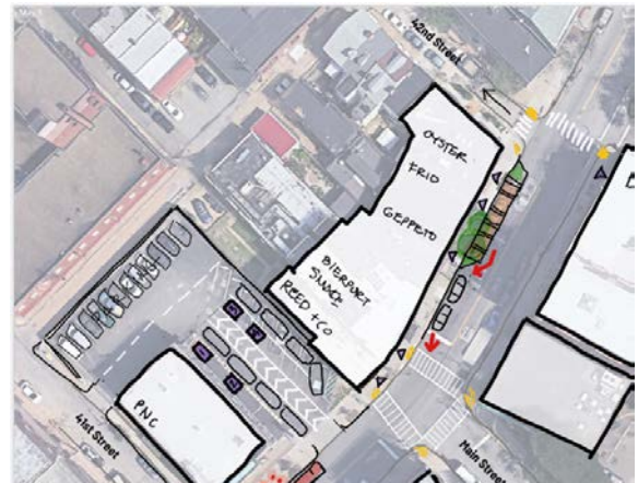
Figure 3: District Approach + Off-street Uses Curbside parking converted to limited seating in front of businesses; bank drive thru converted to efficient curbside pick-up lanes with kiosk outposts from adjacent restaurants; parking lot used for workers; bus stop moved to where wider sidewalks with less competition for space are available. Taken together this keeps sidewalks generally uncongested allowing social distancing; vehicle flow is efficient and easily legible to drivers; transit patrons experience less crowding. (SOURCE: Evolve EA)
