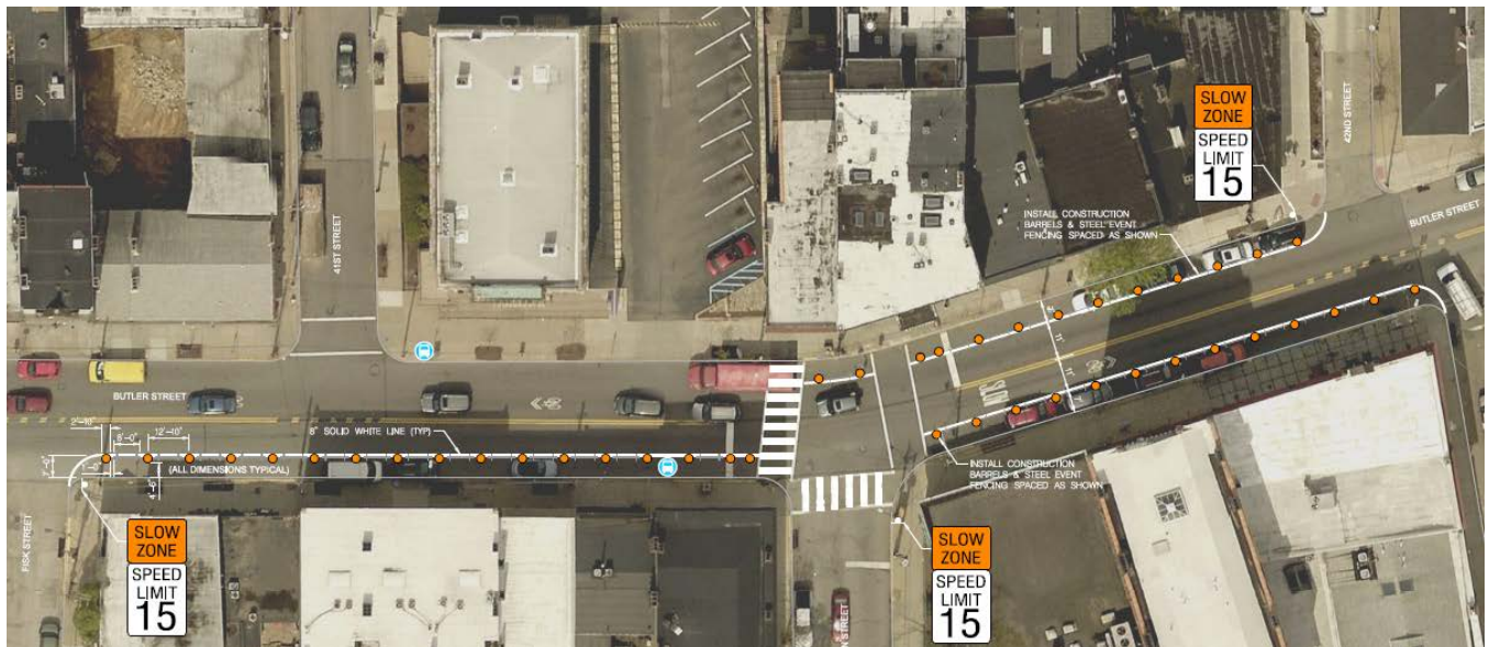
Figure 7 Illustrative redesign of Butler Street using temporary construction zone techniques
