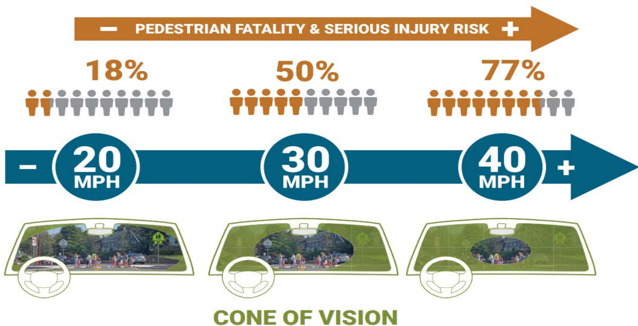
Figure 4 Speed is one of the most consequential considerations in safe redesign (SOURCE: FHWA)
